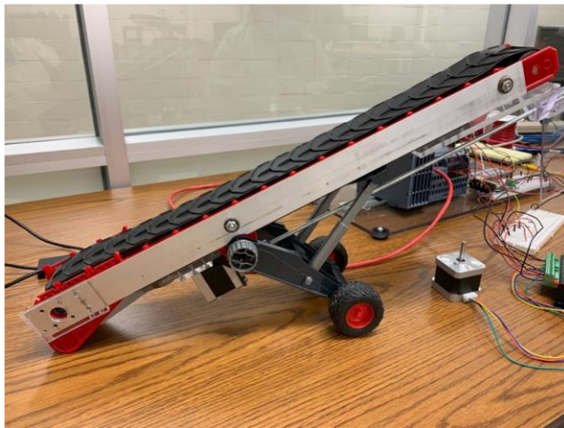
Fig. 7 Conveyor for Chip Sorting
