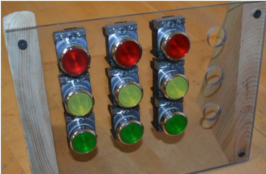
Front side of New Pushbutton Stations
