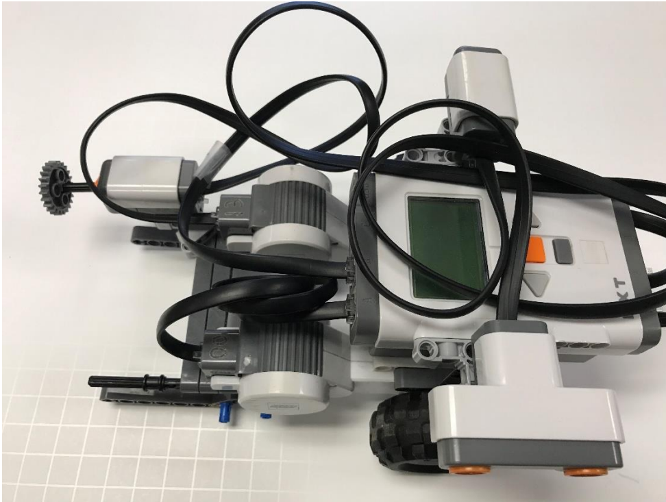
Figure 3.2: Lego Mindstorm NXT robot with Ultrasound ranging sensor (aiming down), a light sensor in ambient mode (aiming up), and a push button (or pressure) sensor facing left.
