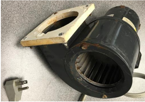
Figure 6.18: Dayton Model 4C446 blower fan that uses a 1/25 hp single phase induction motor.
