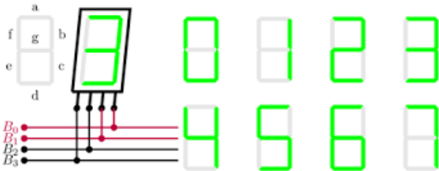
Figure 1.3: A 7-Segment Display to represent an Octal 3-bit symbol (Bit B 3 isn't used). © Germain Gondor. Used under a CC-BY license: http://www.texample.net/tikz/examples/seven-segment-display/
