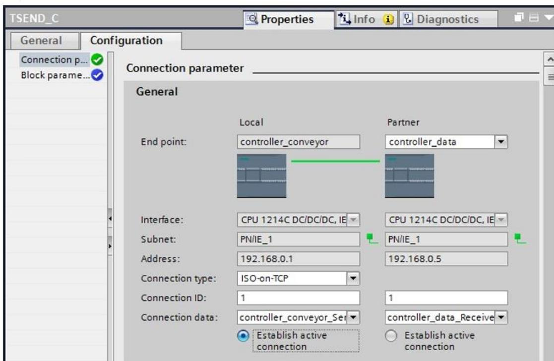
12. The data block is generated and incorporated automatically. Under Properties, select the connection partners. First, at the connection data of the local controller, select the existing data block "controller\_data\_connection\_DB", otherwise, a new data block is generated. Then, select the partner controller and the associated data block.
