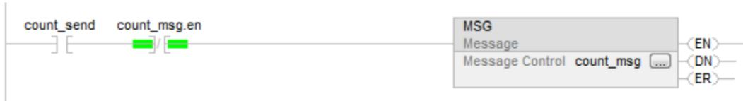
This diagram shows how the controller processes MSG instructions.
