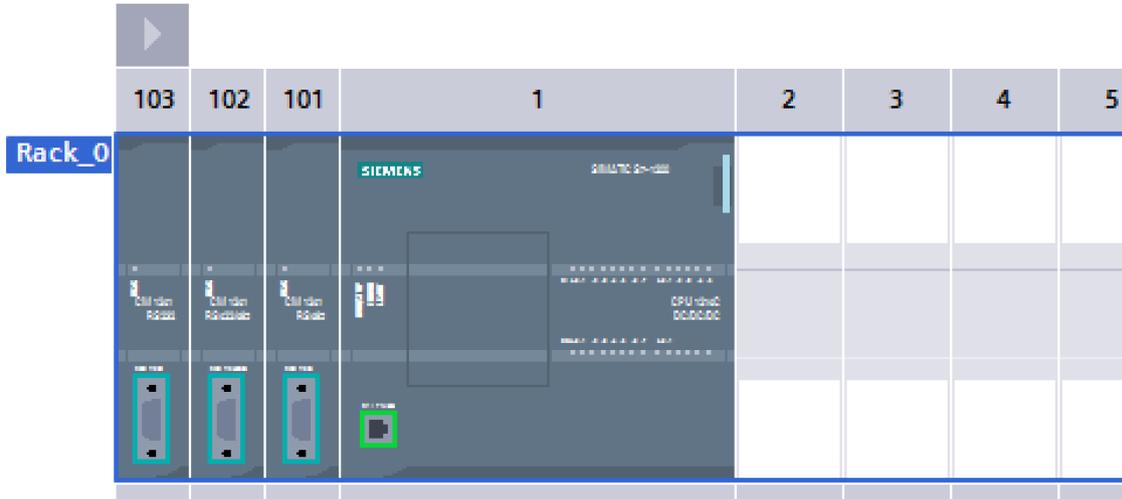
The three cards attached to the left of the CPU in the picture above represent three different configurations of the serial communications port available with the S7-1200 processors. These are the RS-232, RS-422 and RS-485 protocols. Each has a different voltage and current requirement for completion of a data transmission.
