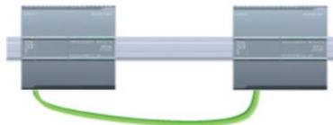
For a direct connection between two CPUs:
