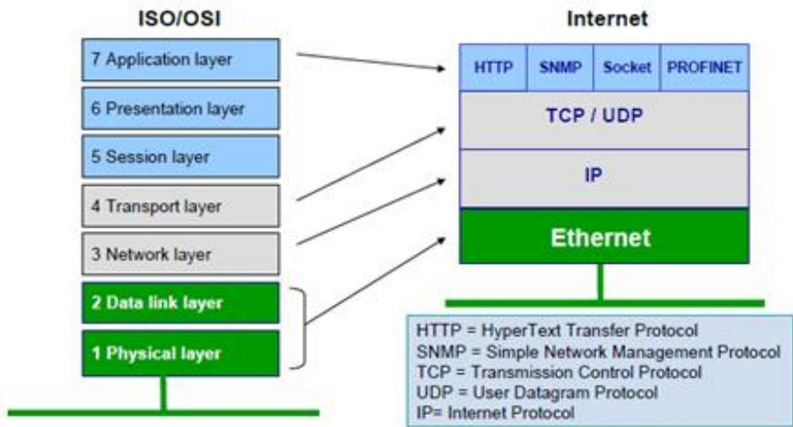
Multiple application protocols can run at the same time on the physical medium (Ethernet)
