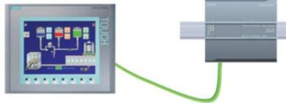
For a direct connection between an HMI panel and a CPU, the project must include both the CPU and the HMI.
