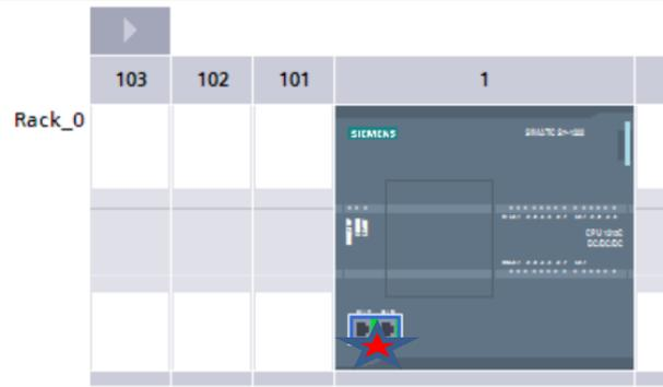
One of the PLCs had to be configured as an IO device which can be seen in the below image. To bring up the menu below I had clicked on the ProfiNet ports shown in the above image.
