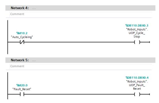
In order to send this information to the robot we need to move the first 2 bytes from DB110 into the LCCF\_EIPScanner block as shown in the image below.
