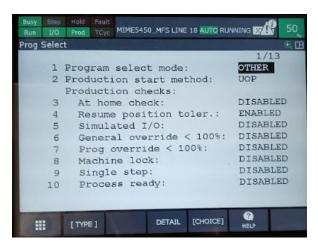
The next step was to add logic to the PLC program to start the robot via the user inputs. In order to start the robot user inputs 1, 2, 3 and 8 need to be on and user input 5 needs to be pulsed on for at least 10ms. I created a separate function call and data block in the PLC to contain this logic. I used
