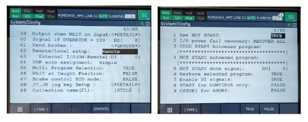
Next, I had to configure the method by which the robot is started. This can be accessed from the Program Select screen on the Teach Pendant by pressing the Menu key and then Setup followed by Program Select. From this screen set the Program Select Mode to Other and the Production Start Method to UOP. With 'OTHER' highlighted press Detail on the pendant. This will display another screen allowing for a program to be selected to run when the robot is started.
