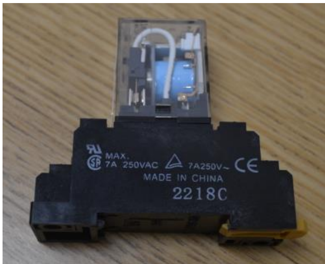
Fig. 2-38 Omron MY2N-D2 Relay
