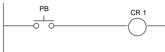
Fig. 2-3 Example of Ladder Logic
