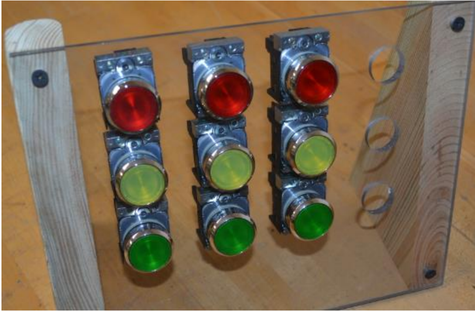
Fig. 2-41 Above – Front side – Below – Back Side of New Pushbutton Stations
