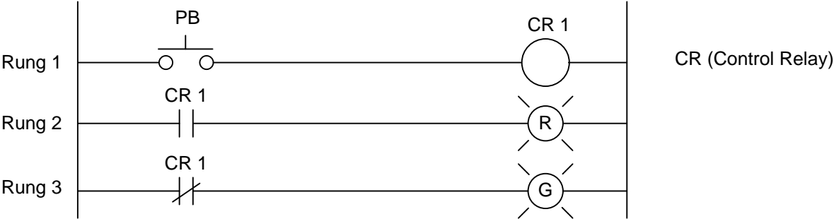
Fig. 2-5 A Control Relay (CR) with various Contacts
