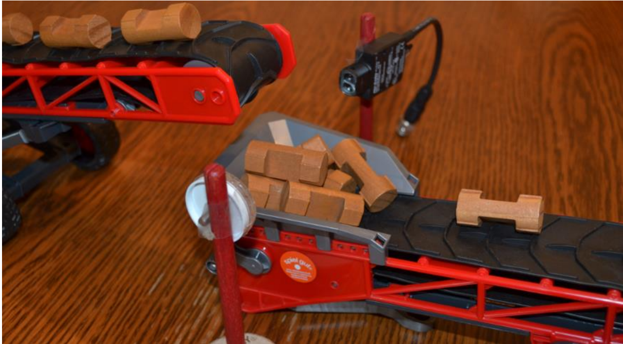
Fig. 7-44a Conveyor Problem with Build-up
