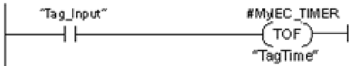
Fig. 7-12 Start Off-Delay Timer Input
