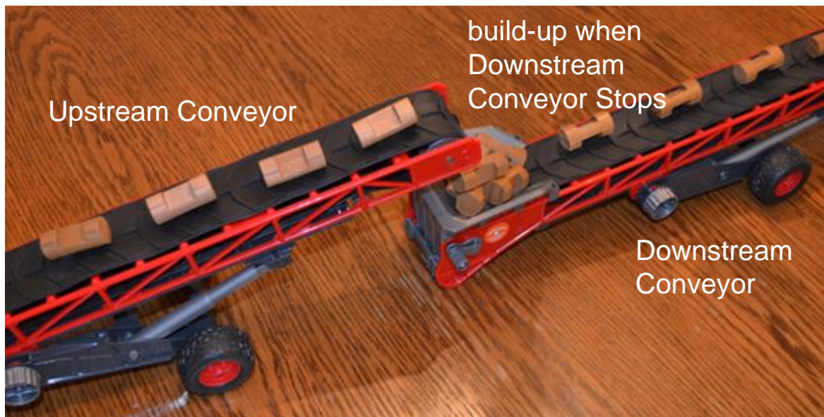
Fig. 7-43 Conveyor Problem with Build-up
