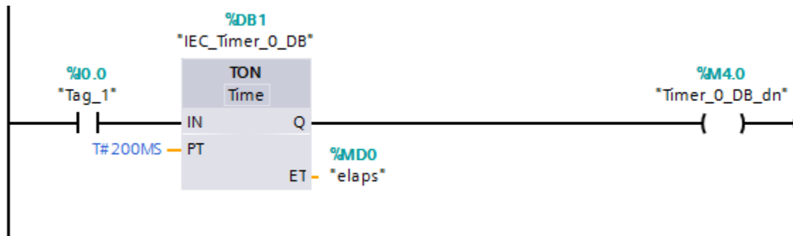
Fig. 7-7 On-Delay Timer Programmed in Ladder
