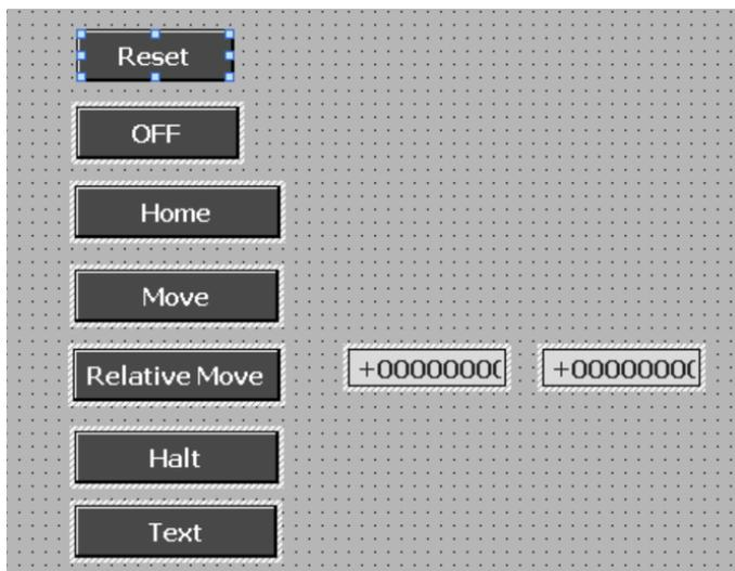
Follow the video from Chapter 17 and build an HMI panel with soft switches similar to the hard-wired switches above. The soft switches provide the same function and should be accessed in the same order listed above to initialize the drive to move.
