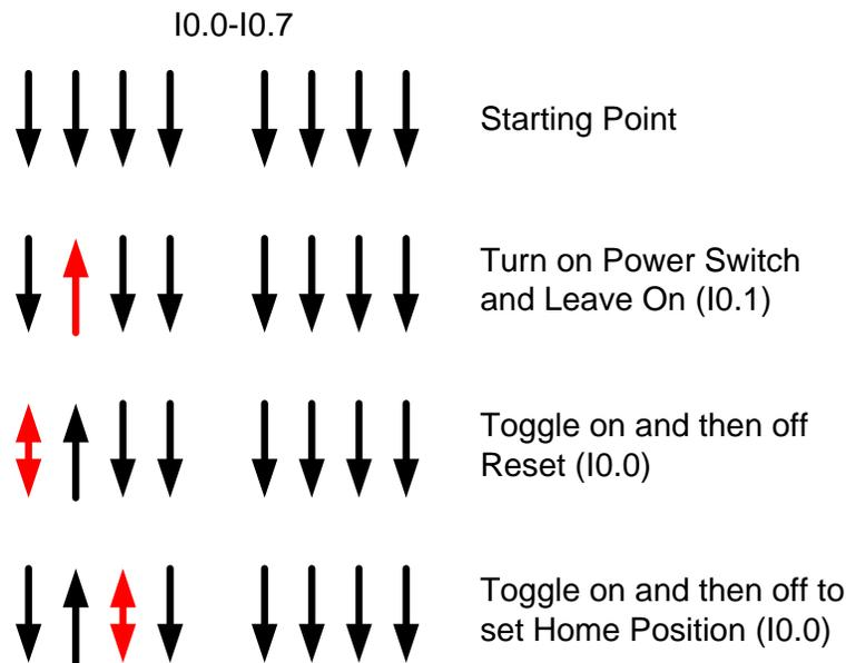
Toggle Switch Settings for Siemens Stepper
