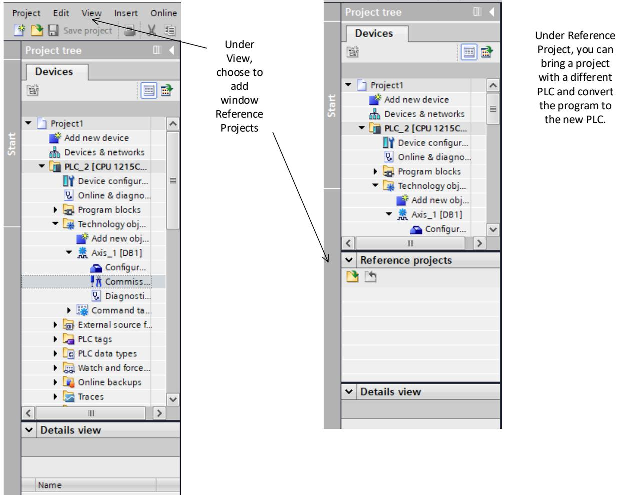
The reference project allows the processor type or version to be changed without change to the program. Otherwise, a number of copy-paste operations are needed to move the contents of one program to another and this process may not change all the variables.
