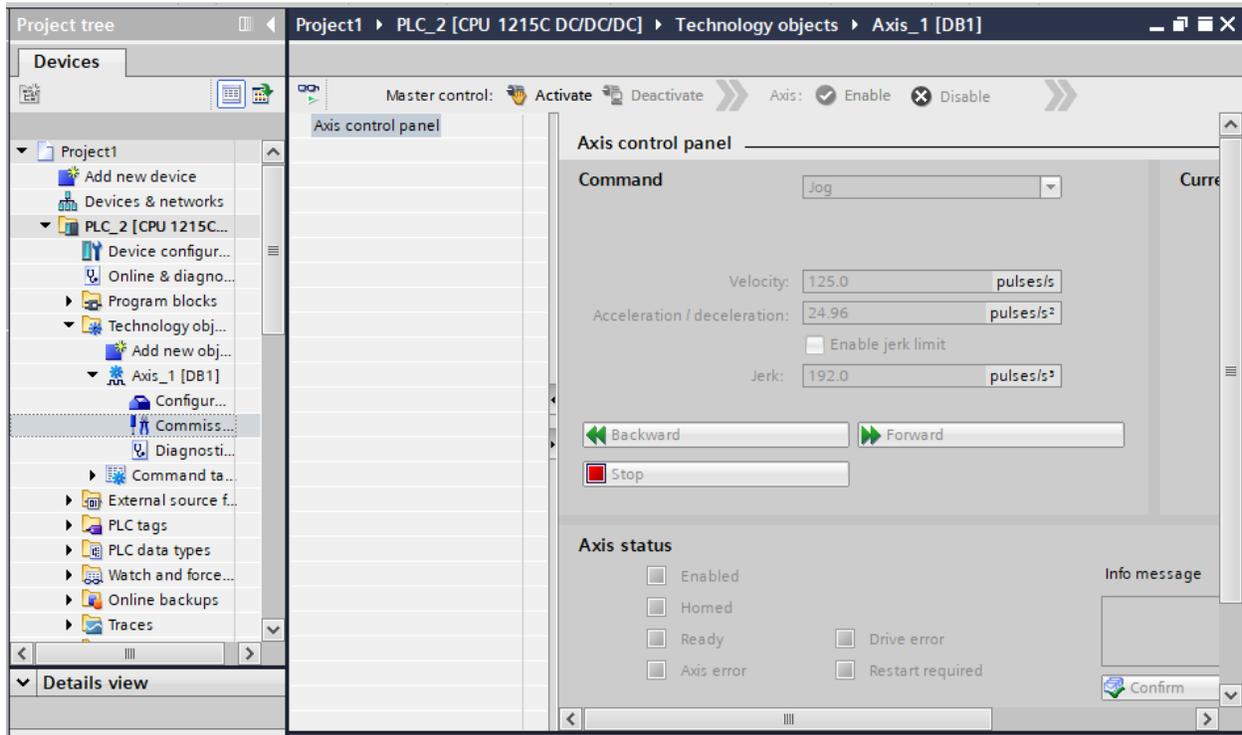
Try Activate, then Enable, and then jog Forward or Reverse. Verify pulses coming from the outputs on the PLC.
