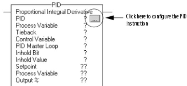
Inclusion of the data tag to create the list shown above. The PID algorithm uses these data tags to calculate and control a PID block. For instance, the PV value for the block is mypid.PV. The SP or setpoint is mypid.SP. The example screens that follow show the newer IF4XOF2F/A card and are used to set up the scaling for the present system in the lab.
