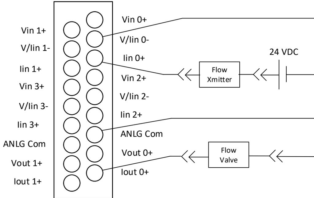
The wiring diagram of the card is shown above. The input and output range of the 4-20 mA engineering units can be found by looking up the accuracy of the signals. Both have a range of 0 mA to 21 mA – 0 to 32640 decimal range. So, 4 mA would be 6217  $(32640/21)*4$  and 20 mA would be 31085. Our range for the raw input and output then is 6217 – 31085.
