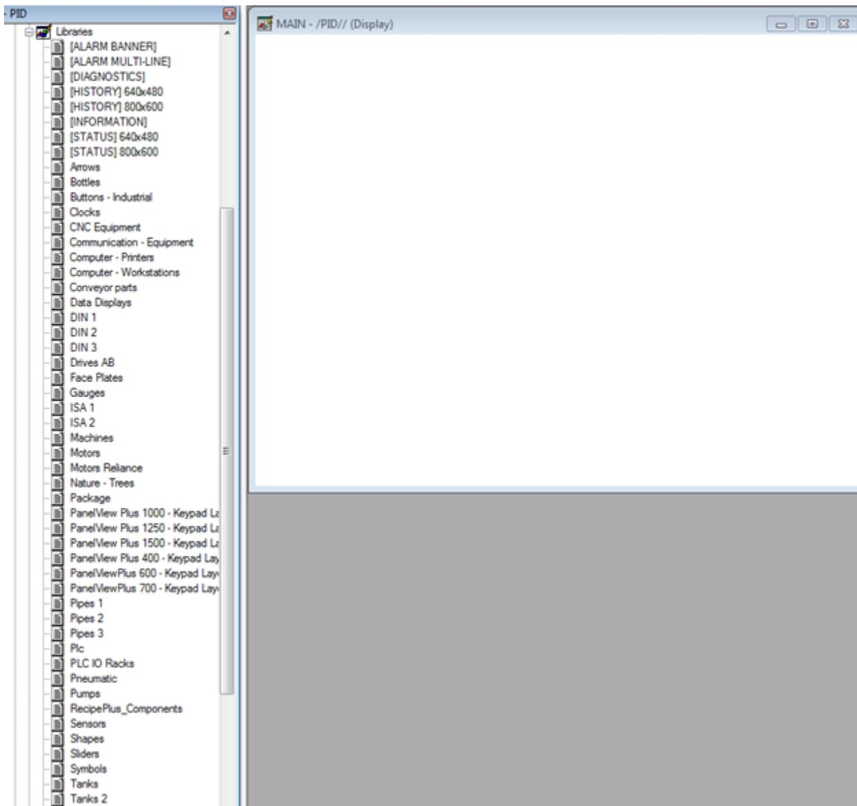
With RSStudio, build a screen from scratch using a face plate. There are a number of face plates in the template from which to choose.
