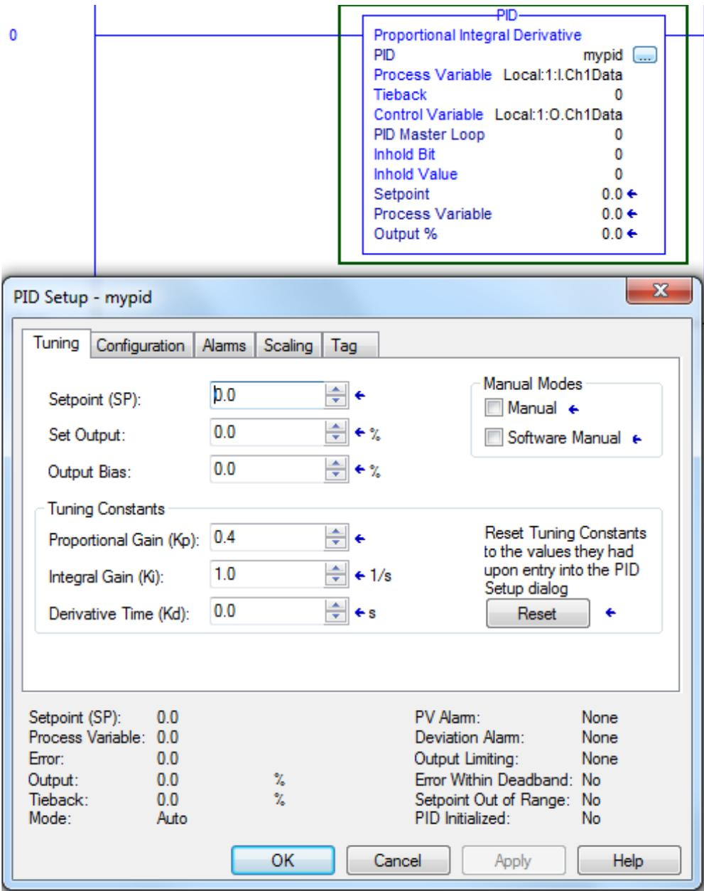
The tuning tab shows the variables used to tune the PID block. The Kp, Ki and Kd tuning constants are probably the best variables for the water valve. These constants should not vary too much from the numbers shown or the PID block may become unstable.
