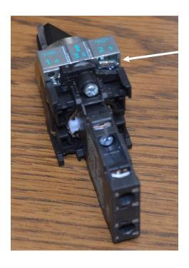
In order to change or move Siemens buttons, simply move the lever to the <u>left</u> as shown. It may not move easily so first you may need to loosen the screw and then move the lever.
