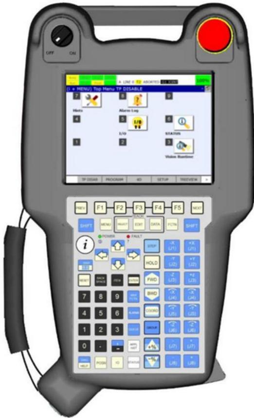
The teach pendant shown at right provides a number of functions for control of the robot including:
