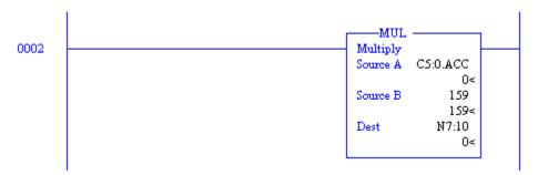
The number in Source B may be either a constant (as is here), or a value from a N7 location. If from an N7 location, the value that is to be used must be entered into that N7 location.
