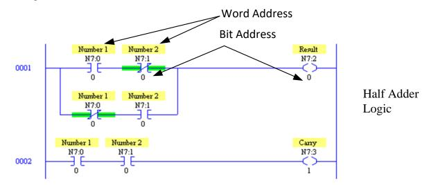
The number in location N7:0 is added to the number in N7:1. The result is stored in location N7:2. The carry is located in N7:3. The same locations are used for remaining bits of the word shown in Fig. 8-36. Full adder logic for each remaining bit from 1 to 15 is required. The logic must be duplicated for each bit. Carry\_In is from the prior bit. The Carry\_In for bit 1 is found in Carry\_Out of bit 0.
