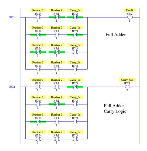
It is worth noting that to actually build this logic requires a great deal of time unless the Copy-Paste function is employed. Once the logic is built, changing the bit numbers in the logic is all that is required for succeeding bits from 2 to 15.
